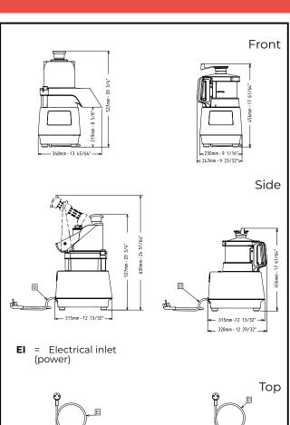
Electric Supply voltage: 220-240 V/1N ph/50/60 Hz **Electrical power max.:** 0.75 kW 0.75 kW **Total Watts:** Capacity: Performance (up to): 150 kg/hour Capacity: 2.6 litres Key Information: External dimensions, Width: 348 mm External dimensions, 315 mm Depth: External dimensions, Height: 527 mm **Shipping weight:** 22.2 kg
